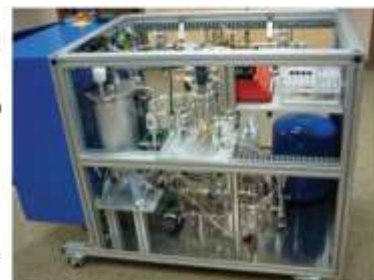
Early Warning's analyzer feeds a concentrated water sample to its biosensor, providing rapid pathogen detection
